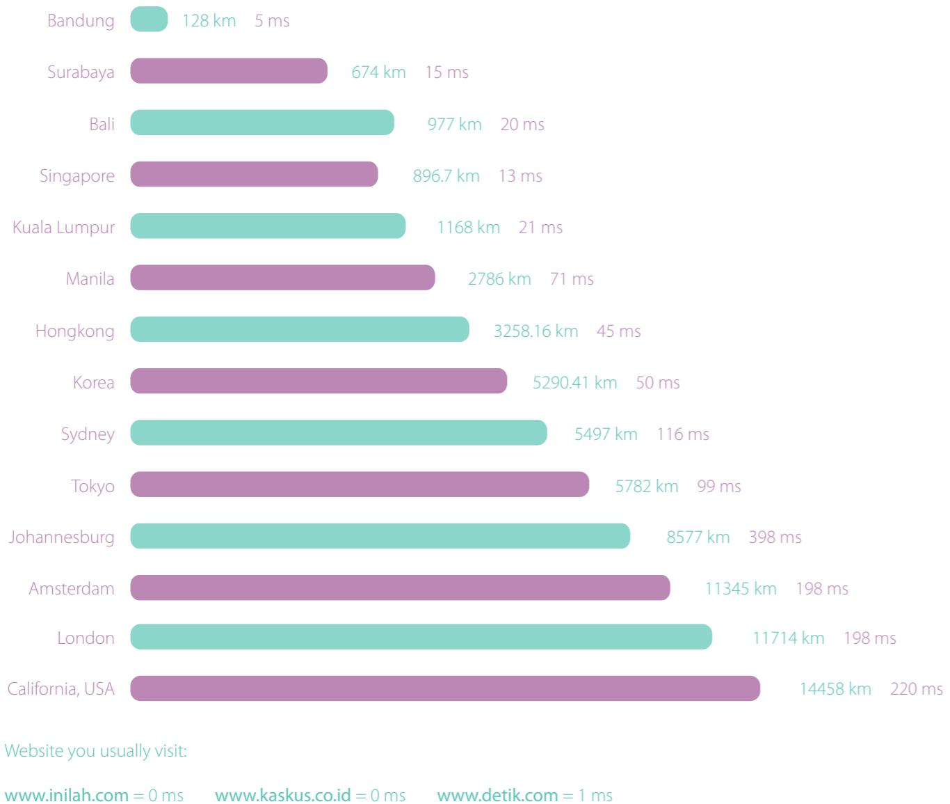
Ping times above are the average of total time spent in reaching the destination from your computer through Biznet Network in normal condition. Ping time indicated in milli-seconds (ms), 1 ms = 1/1000 second
